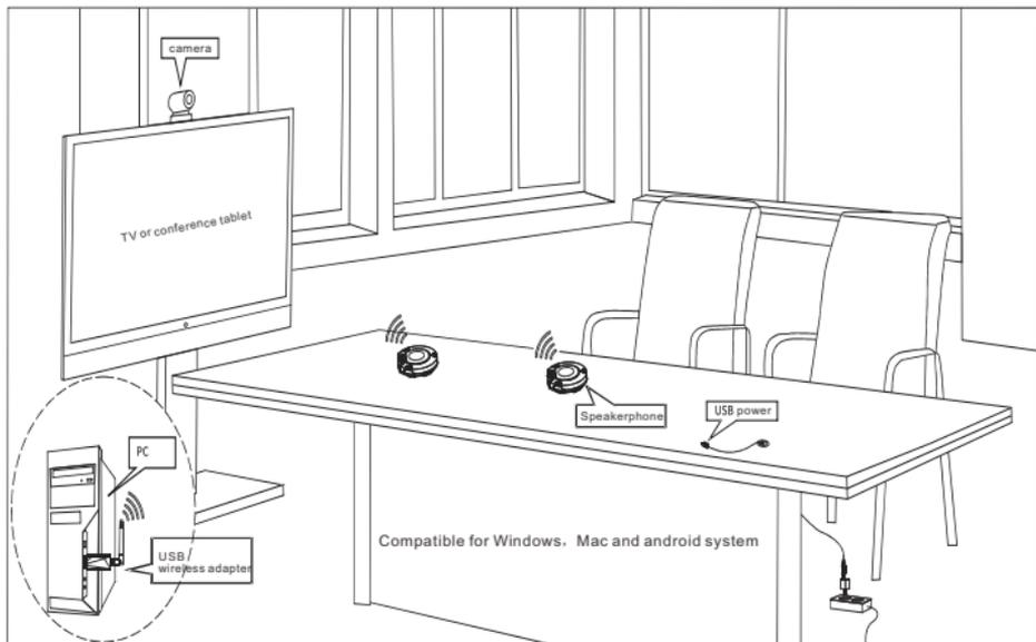
Note: do not place the device host within 10cm of the 2.4g wireless adapter. When it is less than 10cm, there may be no sound pickup and abnormal use.
